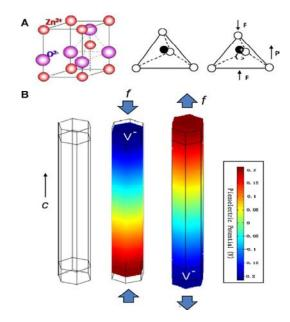
Figure 1. Piezopotential in wurtzite crystal. (A) Atomic model of the wurtzite-structured ZnO. (B) Numerical calculation of the piezoelectric potential distribution in a ZnO nanowire under axial strain. The growth direction of the nanowire is c-axis. The dimensions of the nanowire are L = 600nm and a = 25 nm; the external force is fy =80nN [9].
