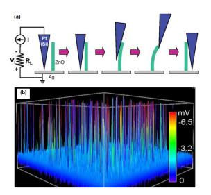
Figure 2. (a): Experimental setup and procedures for generating electricity by deforming a PZ NW with a conductive AFM tip. The base of the NW is grounded and an external load of RL is applied. The AFM scans across the NW arrays in contact mode. (b) Corresponding output voltage image of the NW arrays [7].
