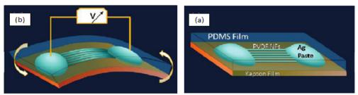
Figure 7. (a) The PVDF NF lies on a Kapton substrate, with both ends bonded with silver paste and the entire device encapsulated with PDMS. (b) Mechanical bending of the substrate creates tensile strain and a corresponding piezoelectric field along the fiber that drives the electrons through an external load back and forth following the cycled mechanical action [21].
