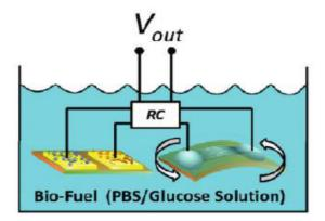
Figure 8. Schematic of biomechanical and biochemical hybrid energy harvester [21].
